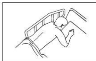
Zone 3: Between the rail and the mattress
